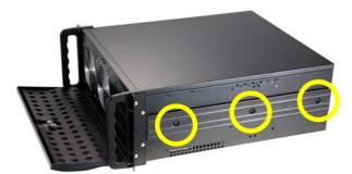
In order to install the rail, you must first remove the cover on the side. Three screws locate on each side.
